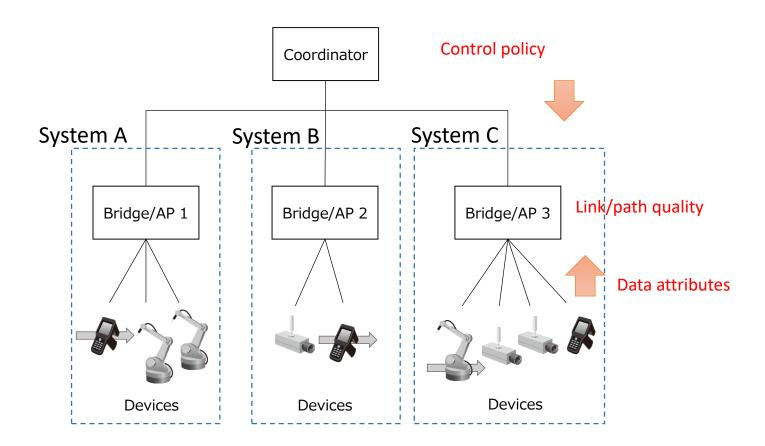
Each system operates autonomously to adapt to short-term fluctuation of wireless links.
