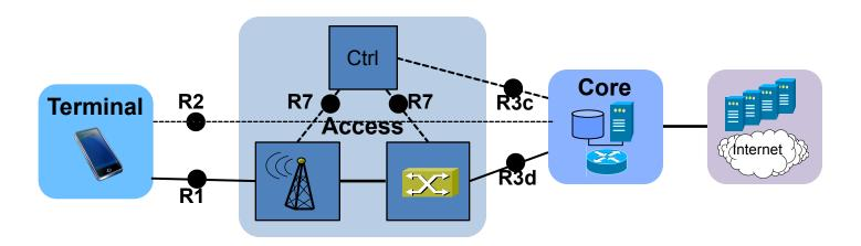
Note: Compatible with model from omniran-14-0051-01; no reference point between backhaul and access point.
