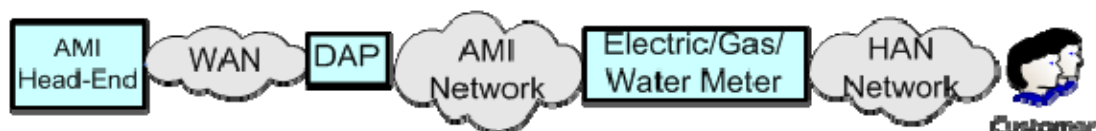
Figure 2: High level example of an AMI system
