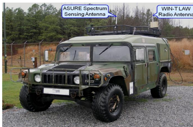
Figure 1. PM C4ISR-OTM vehicle containing an ASURE node consisting of a WIN-T LAW radio, external sensing and cognitive engine software
