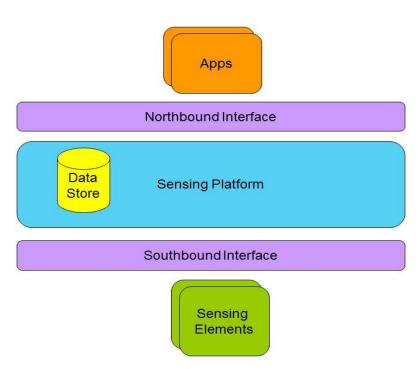
The above block diagram shows spectrum sensing platform that provides spectrum sensing service for various potential applications. The sensing platform defines two interfaces: (A) South-bound interface to the sensing elements or spectrum sensing device (SSD) (B) North-bound interface to the 'Apps' using the services provided by the sensing platform.
