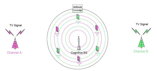
Whenever CPEs in a group detect the re-appearance of a Primary signal (TV signal), BS will turn off communication over that channel and will switch to another available channel. The detection and false alarm probability in this protocol depends on the number of active CPEs.
