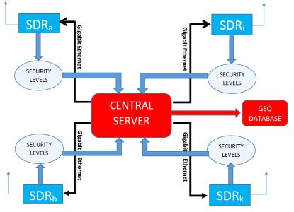
In phase 2, SDRs perform sensing according to the received parameters and additional information consisting of time-stamp, task execution time and GPS coordinates is provided together with occupancy data.
