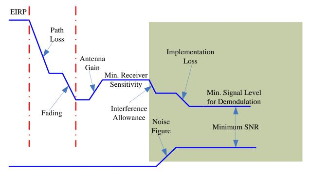
Thermal Noise Floor = -174dBm/Hz +  $10\log(BW) = -106.2$  dBm for 6 MHz TV band
