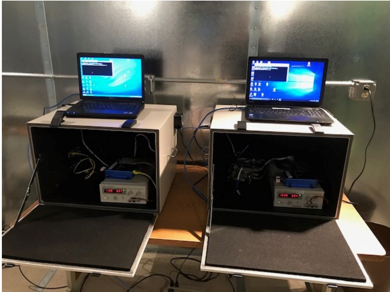
Figure 213 – U-NII-4 and DSRC test setup with DSRC devices inside RF enclosures
