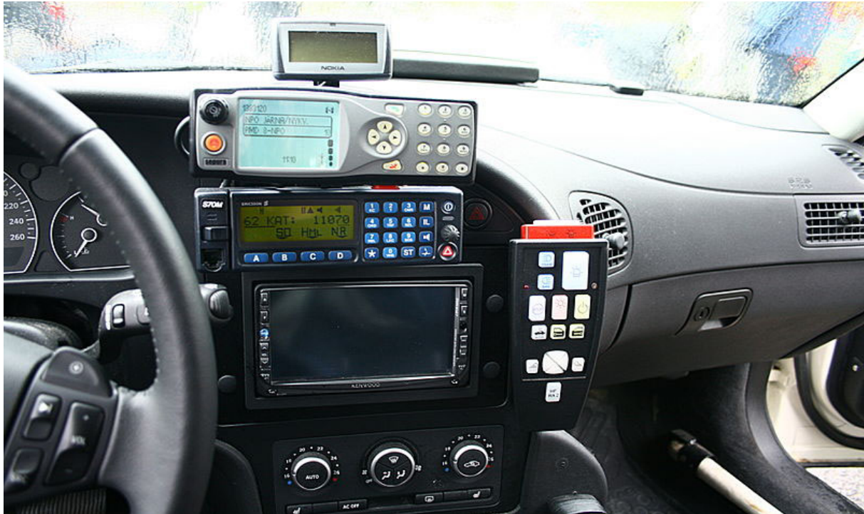
Figure A.4. Swedish police car with RAKEL (TETRA) transceiver above a still-used older radio system's transceiver and a digital video monitor
