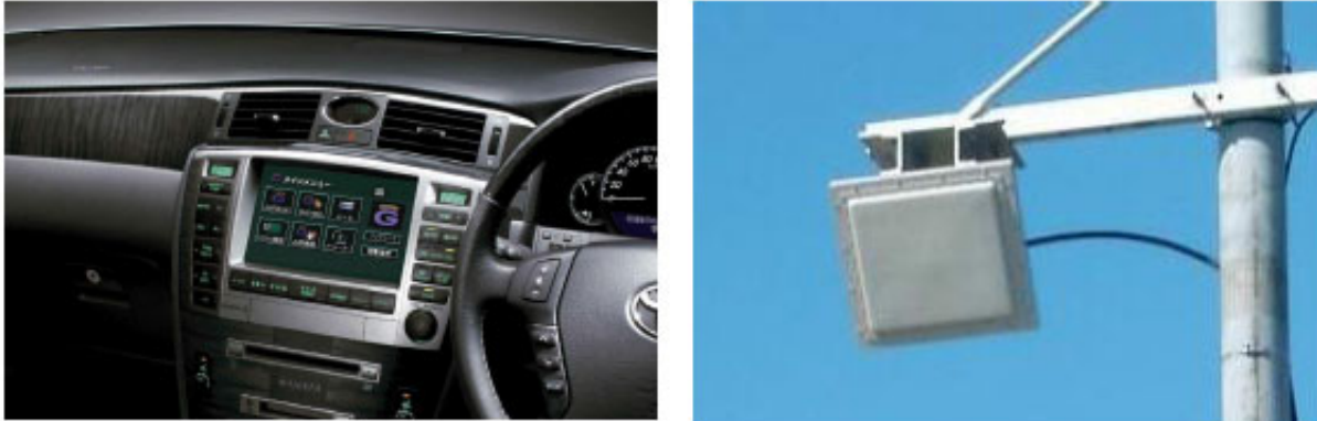
Figure 5.4. ITS Spot-compatible car navigation system (left) and ITS Spot roadside transceiver (right)
