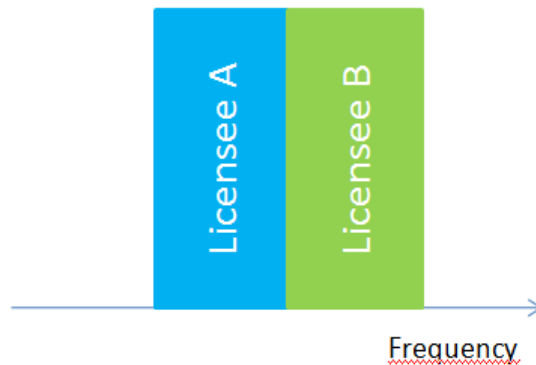
Figure 19: Licensing situation for two adjacent frequency blocks
