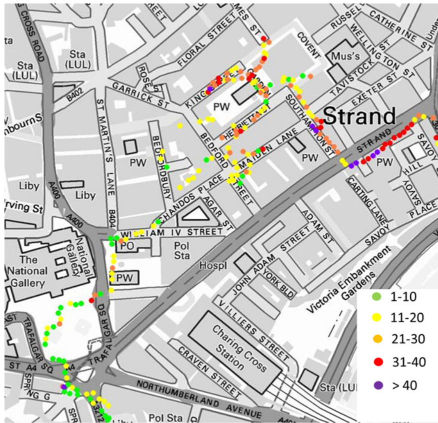
Figure 5-1 Number of access points detectable outdoors at various locations around Covent Garden, London
