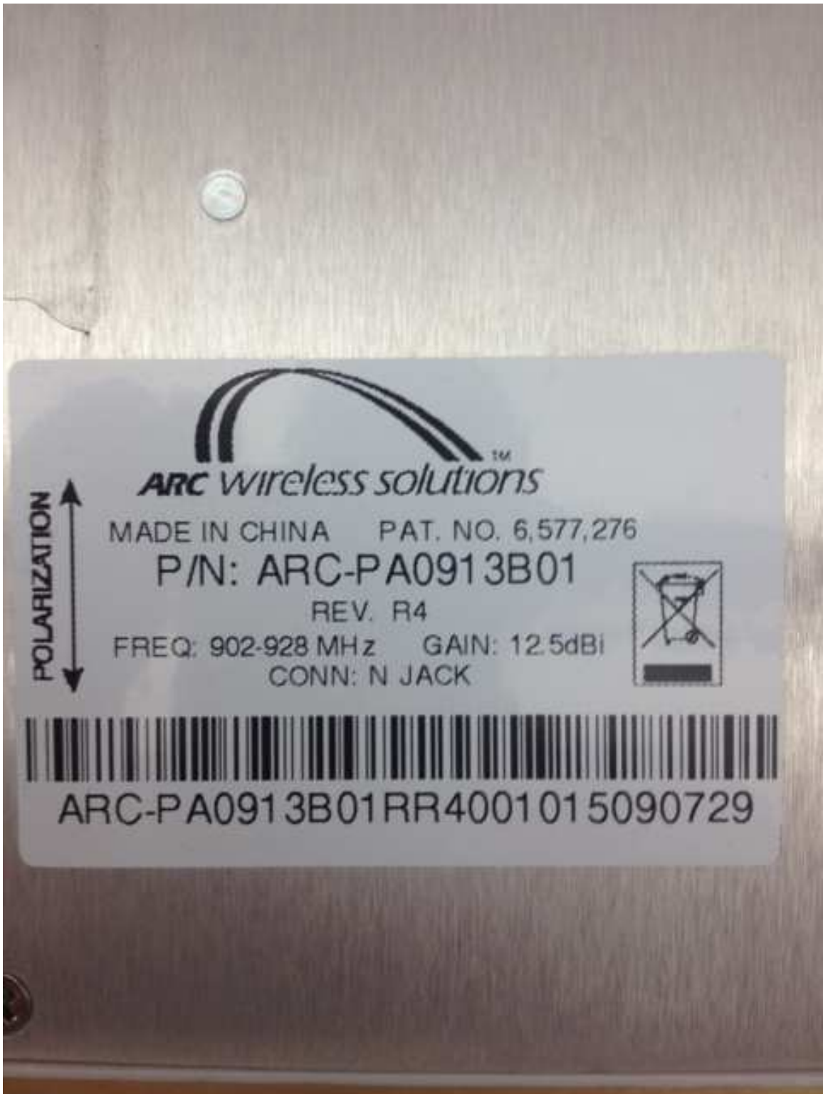
Figure 18: ARC Wireless Antenna used for Canopy AP
