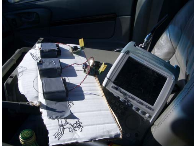
Figure 11. Three Nordic nRF2401 devices operating inside a passenger car at Hooper Island, Maryland.
