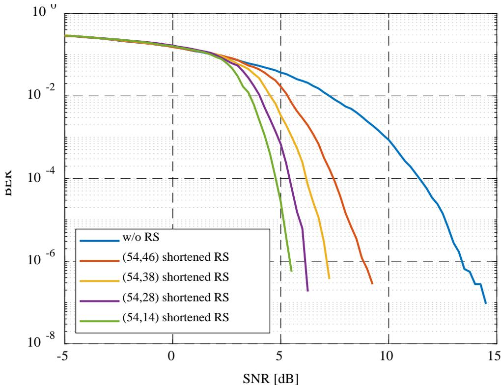
Bit error ratio of (54,46), (54,38), (54,28), (54,14) shortened RS codes and no encoding were evaluated under an AWGN channel and BPSK modulation
