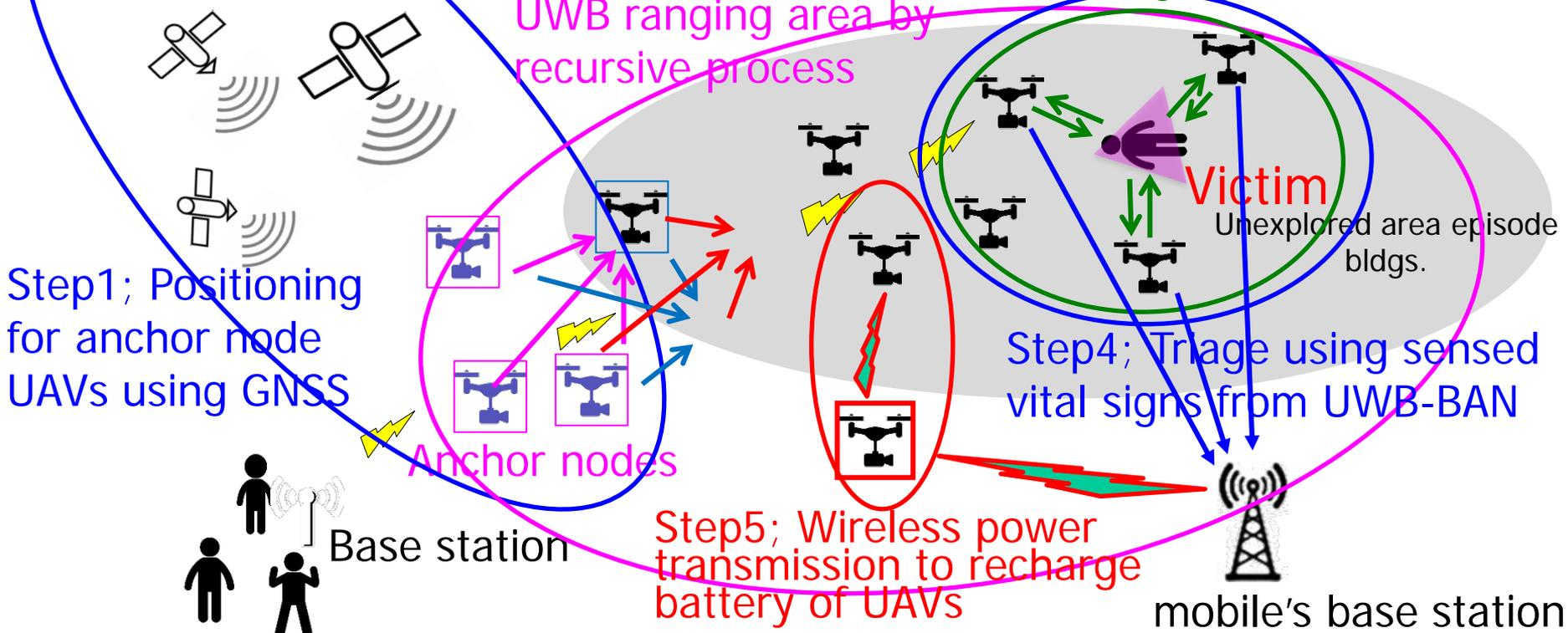
Step1; Positioning for anchor node UAVs using GNSS
