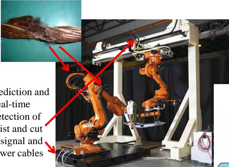
Prediction and Real-time Detection of twist and cut in signal and power cables
