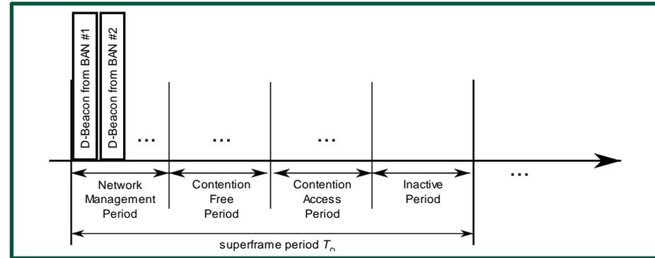
Frames for both Control Channel and Data Channels are accommodated into one single channel.
