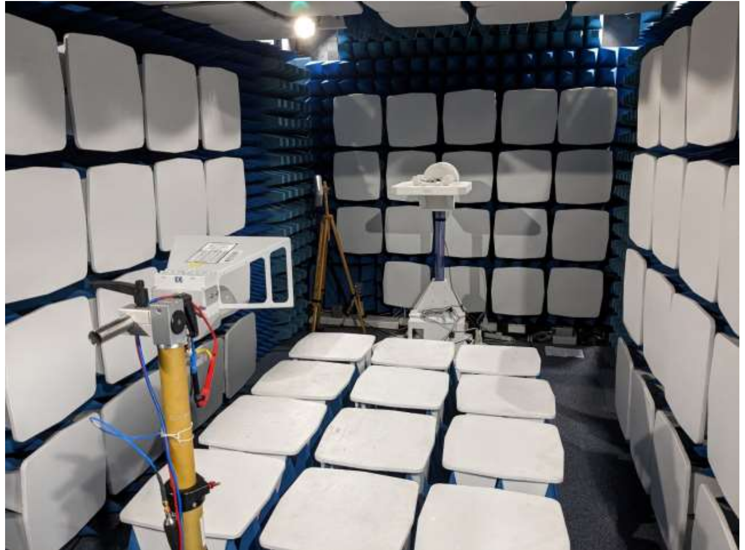
Figure 1: Over The Air (OTA) measurement set up in the Shielded Anechoic Chamber (SAC) in full anechoic configuration.
