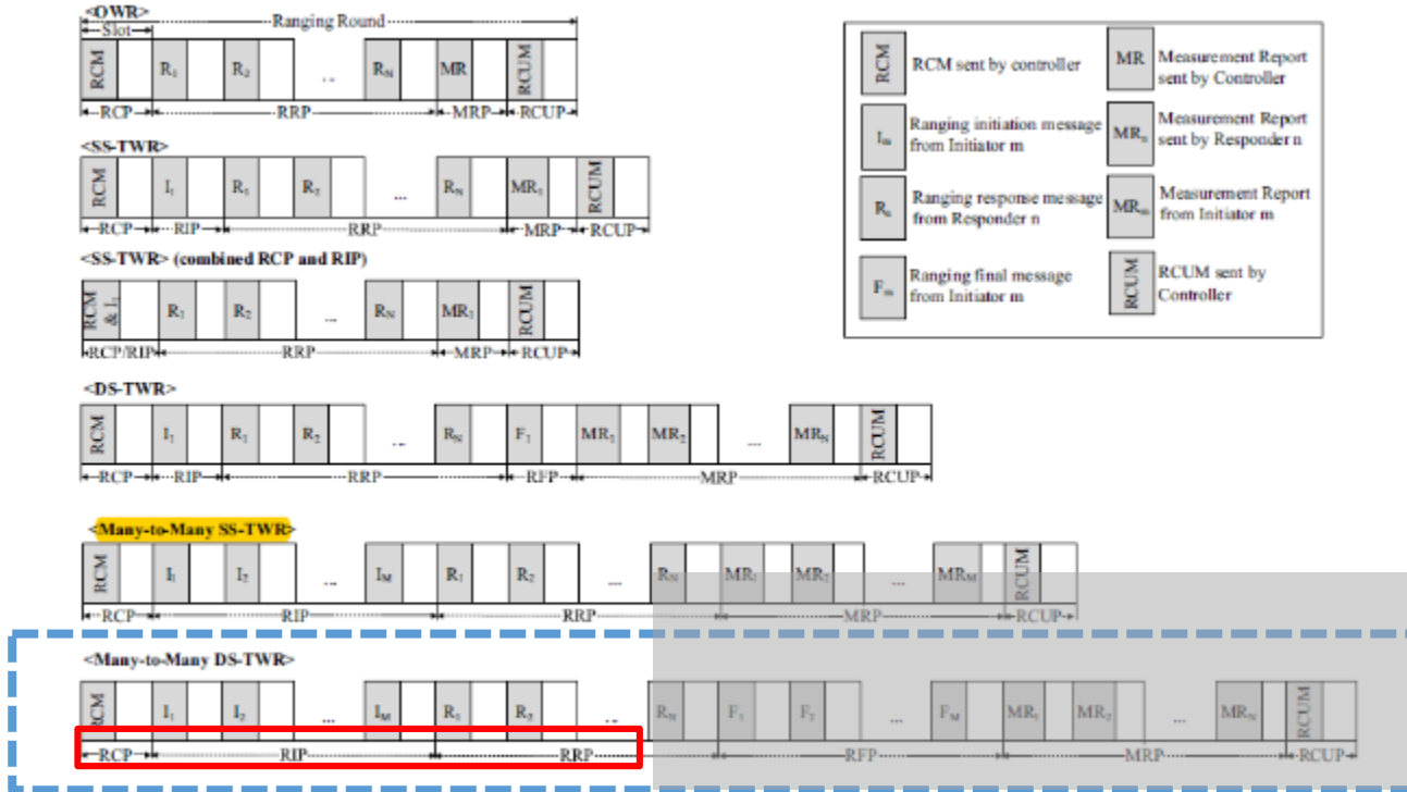
Figure 6-48I—Example timing diagrams for some different multi-device ranging use cases
