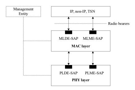
Figure 2—P802.15.6a protocol stack.
