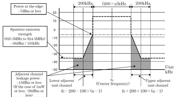
(Note: Center frequency is one of frequencies shown in Table 3.11 to Table 3.15 of 3.2.3 Radio channel and n is a number of unit radio channels constructing a radio channel.)
