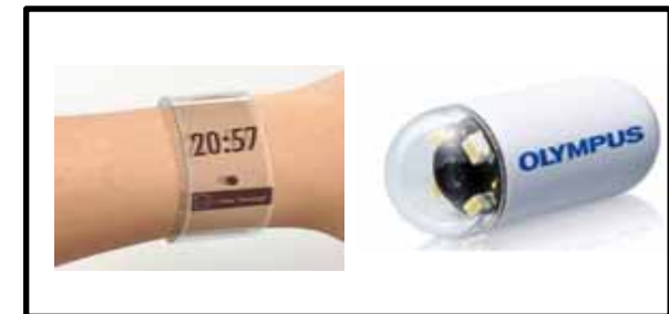
Fig.2 Implanted Wireless Capsule Endoscope
