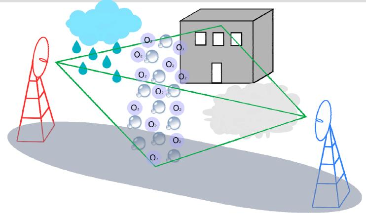
Path Loss / dB = 92.4 + 20 log( r/km) +20 log( f/MHz) + ( $\gamma_0 + \gamma_w + \gamma_R + \gamma_c$ ) r/km
