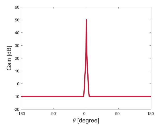
A simplified radiation pattern of 50 dBi antenna
