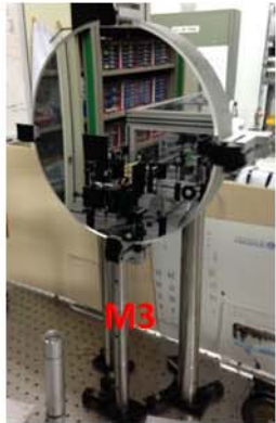
Telescope mirror: 30.5 cm dia. 317.5 cm focal length
