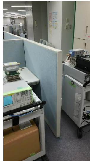
Partition (Thickness is 60 mm) Loss = 22.7 dB
