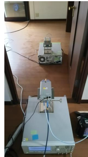
Wooden door of the Wooden house (Thickness is 38 mm) Loss = 12 dB
