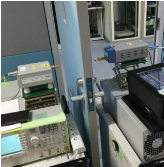
Door (Thickness is 41 mm) Loss = 47.7 dB
