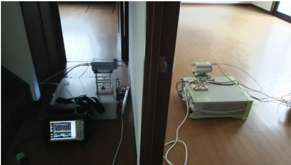
Inside wall of the wooden house (Thickness is 100 mm) Loss = 38.3 dB
