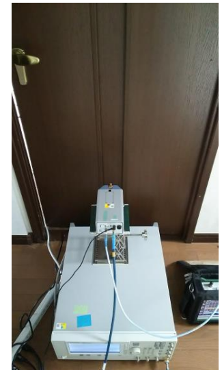
Wooden door of the Wooden house (Thickness is 38 mm) Loss = 12 dB
