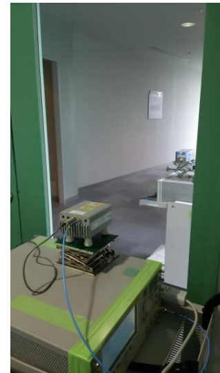
Inside Glass Door (5 mm thickness) Loss = 46.5 dB
