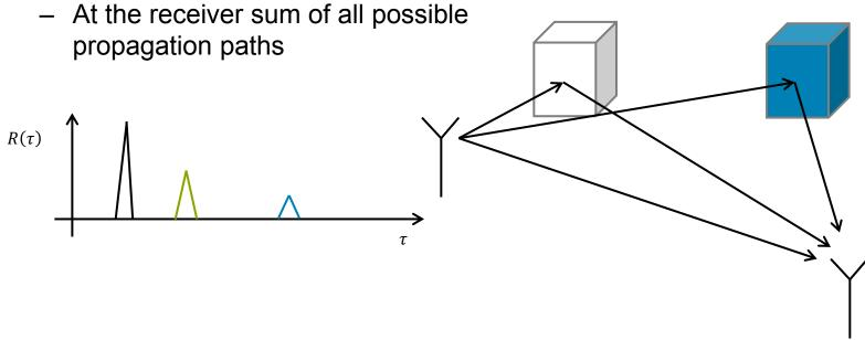
Cross Correlation of received Signal and ideal M-sequence (width of peaks is usually smaller than resolution)
