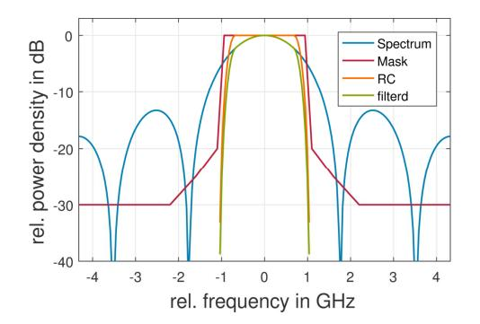
Multiplication of the filter transfer function (RC) with the signal spectrum fulfills the spectrum mask.
