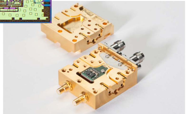
Fully integrated 300 GHz transmitter & receiver MMICs
