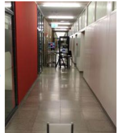
Setup for the world record of wireless data transmission at 100 gigabits per second: The receiver unit (left) receives the radio signal that is recorded by the oscilloscope (right). (Photo: KIT)
