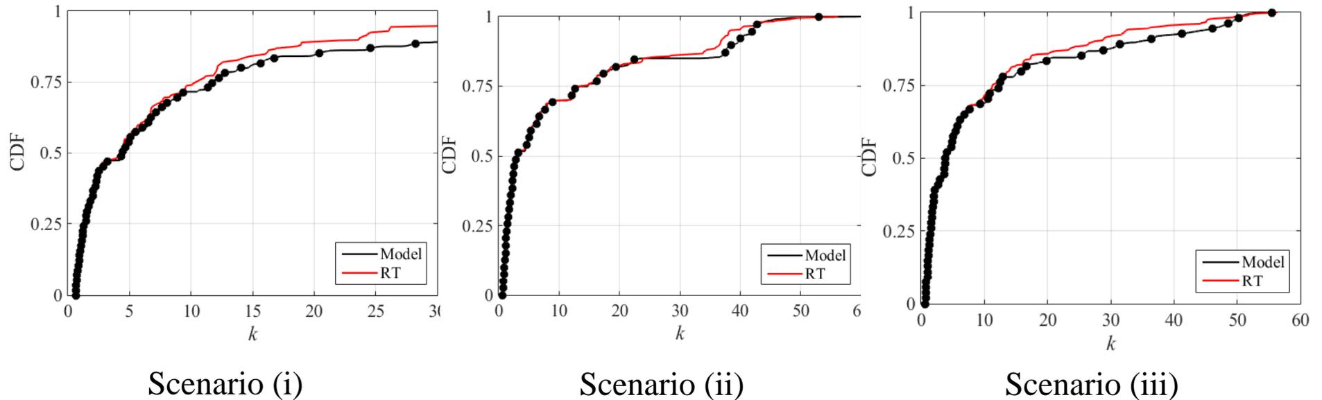
The distribution of K factor of model matches well with that of RT simulations
