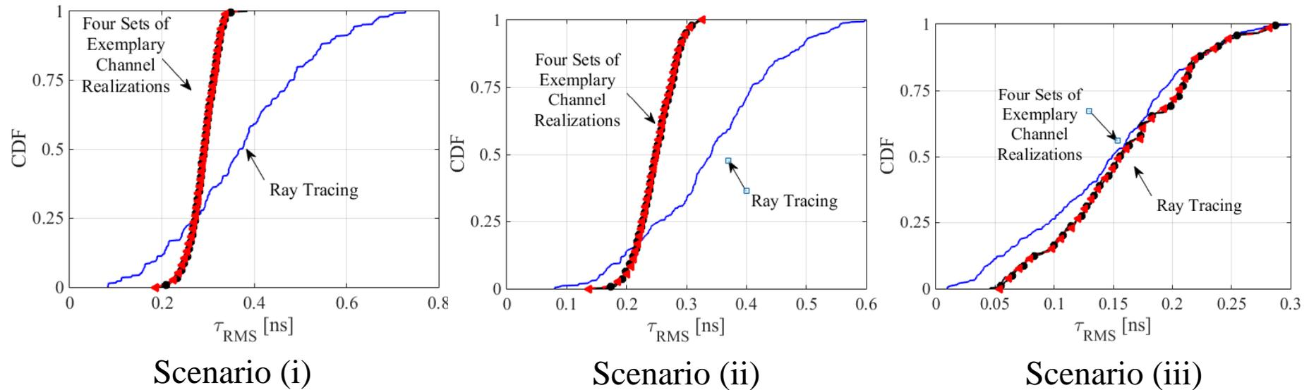
The distribution of RMS delay spread of model matches well with that of RT simulations
