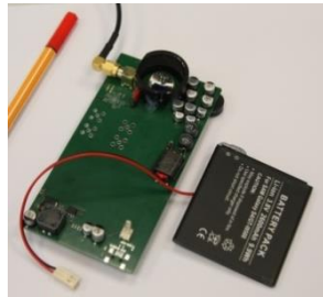
Large-area silicon PD Rx, low cost
