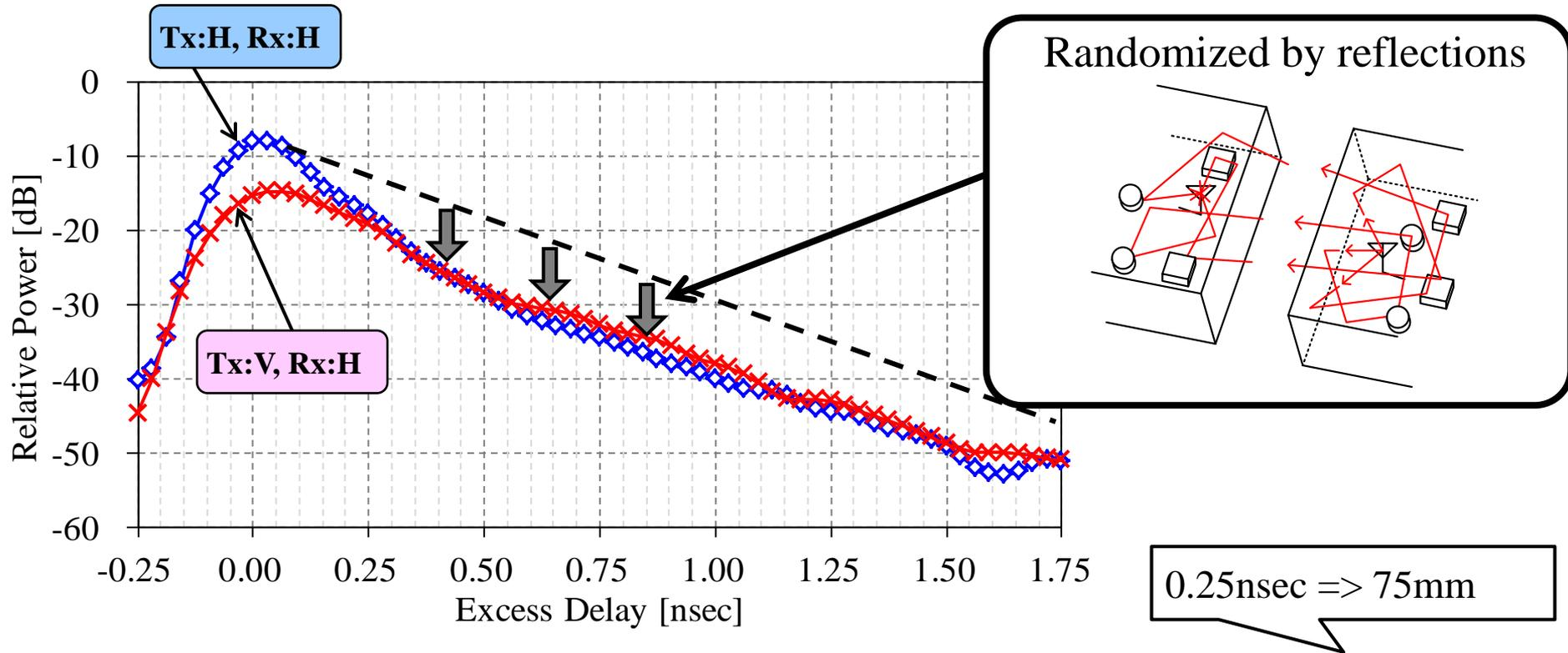
PDP Gap exists on the first path. Two PDPs converge over 0.25nsec.
