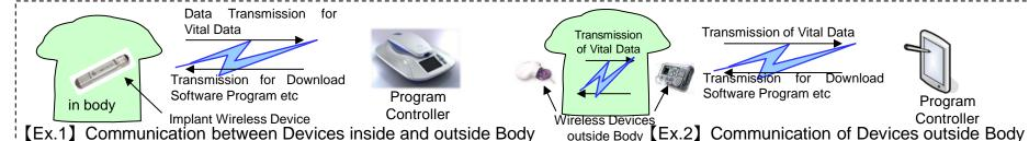
Specified low power radio systems, i.e. current Medical Implant Communication System(MICS) and Medical Implant Telemeter System(MITS) are communicate system between implant medical devices such as pace maker, ICD, vital sensors and devices outside body. On the otherhand, MEDS is a wireless data transmission system between devices inside and outside a body or, one between devices outside a body..
