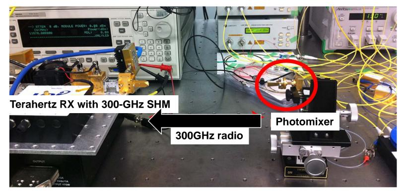
For proof-of-concept demonstration, short-distance transmission was performed because the output RF power of the photomixer was much less than 100 uW.
