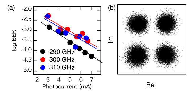
• Power penalty of observed BERs is caused by the frequency response of a photomixer and an SHM.
