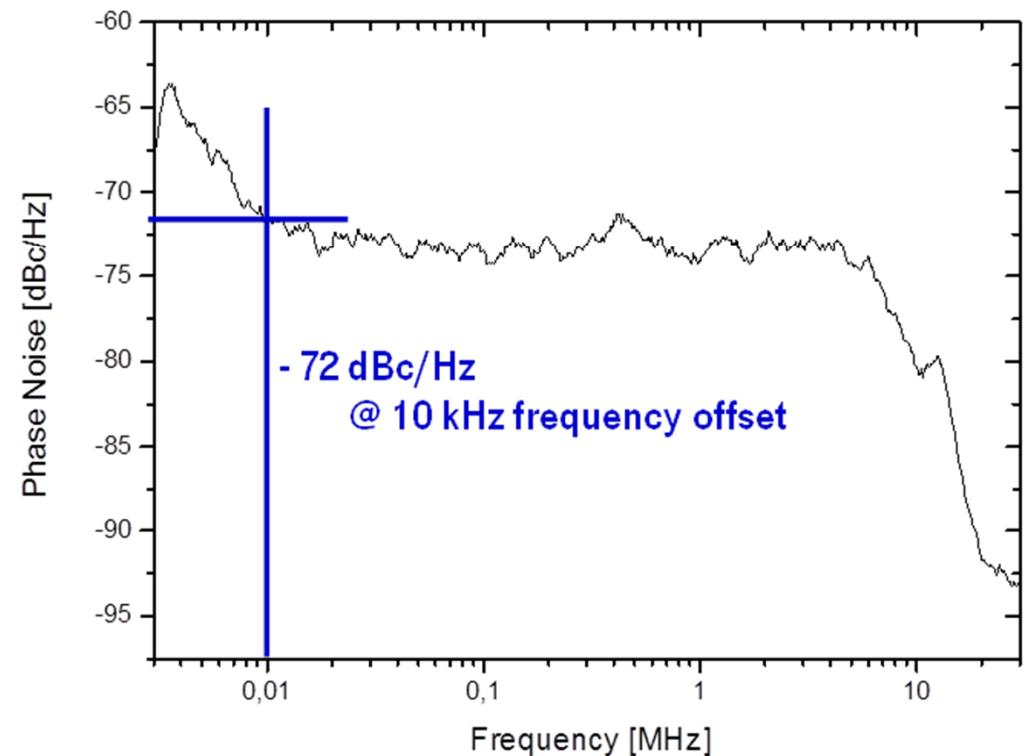
Generated mm-wave measured with an external electrical mixer at the ESA. Therefore the resolution bandwidth is restricted to 300Hz. The right figure shows the according phase noise measurement.
