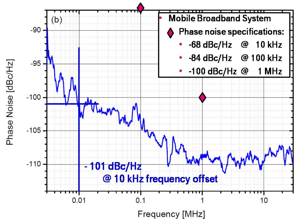
Generated millimeter-wave signal with a frequency of 110.39044 GHz. The measured line-width was restricted by the resolution bandwidth of the ESA due to the used microwave mixers (<300 Hz). In (b) the phase noise measurement is shown.
