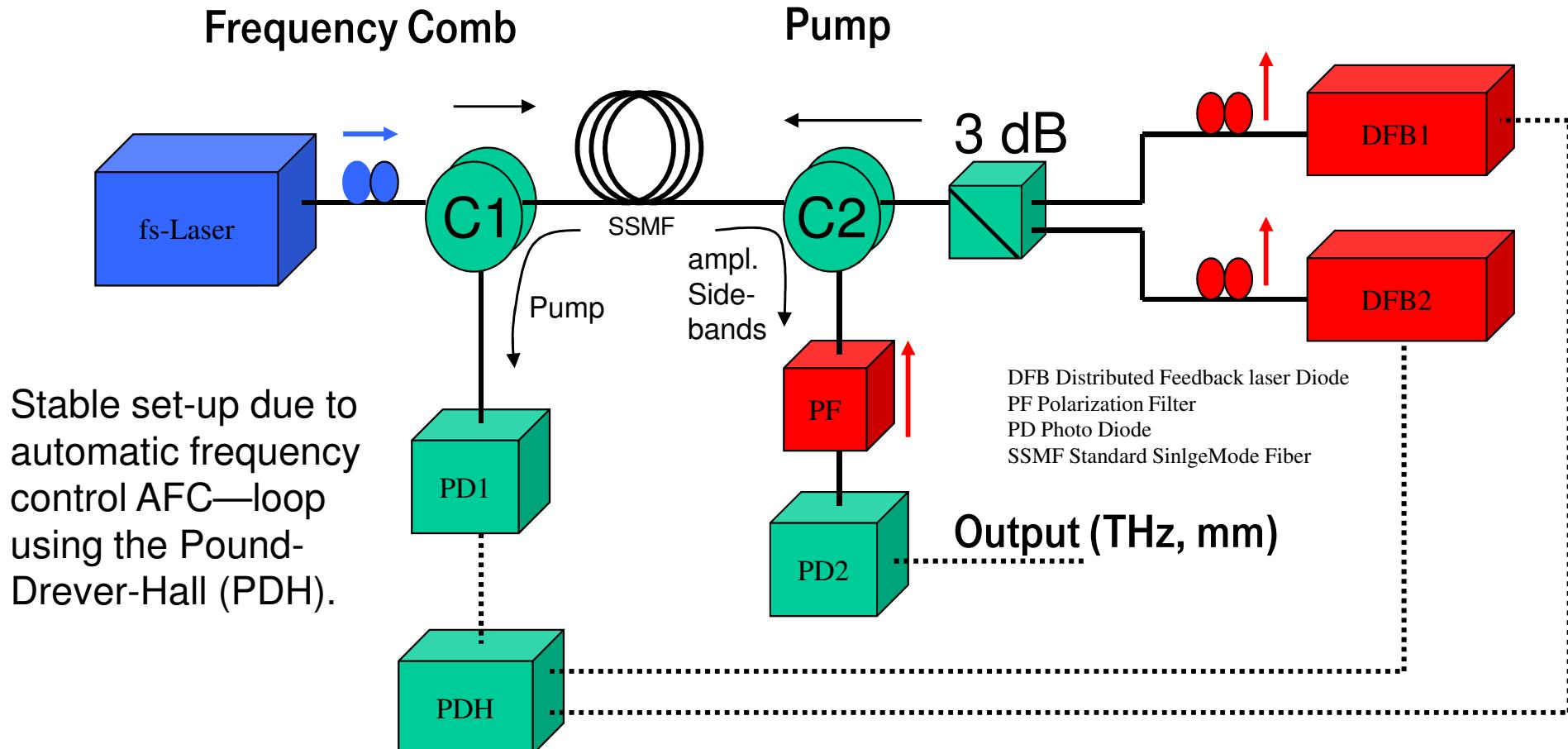
Optical small bandwidth amplification of two selected optical comb lines using the polarization assisted Stimulated Brillouin Scattering (SBS) gain of counter-propagating optical waves.
