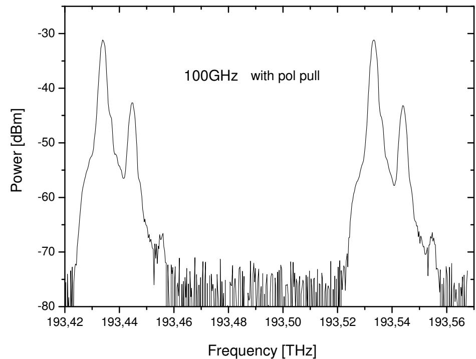
Amplification of two modes out of the spectrum of the fs-laser. There are 1342 modes between the two amplified ones. The remaining modes are suppressed due to the polarization pulling characteristics of SBS.
