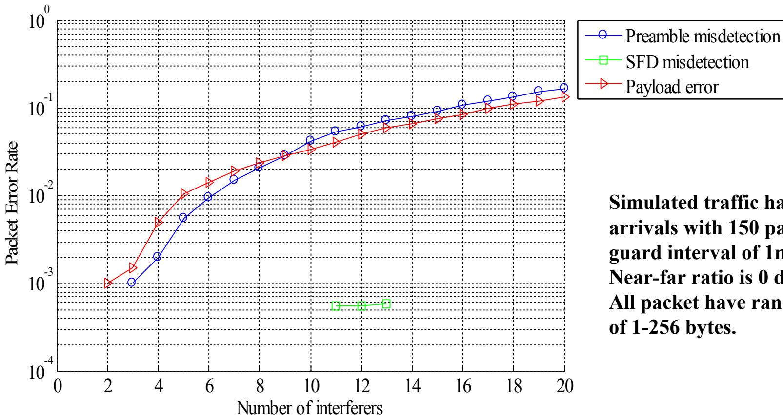
**Simulated traffic has Poisson arrivals with 150 packs/s and guard interval of 1ms.
