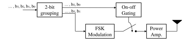
b<sub>1</sub>: conveyed by the conventional FSK-modulated signal
