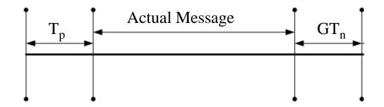
T<sub>p</sub>: Propagation delayGT<sub>n</sub>: Nominal guardtime
