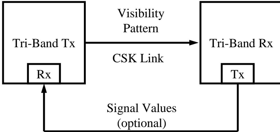
**Figure 1** – Control loop for a color-stabilized CSK link. The calibration sequences are discussed in detail in Section 4. The back link used for routing the compensation factors back to the tri-band Tx does not need to be a CSK link.
