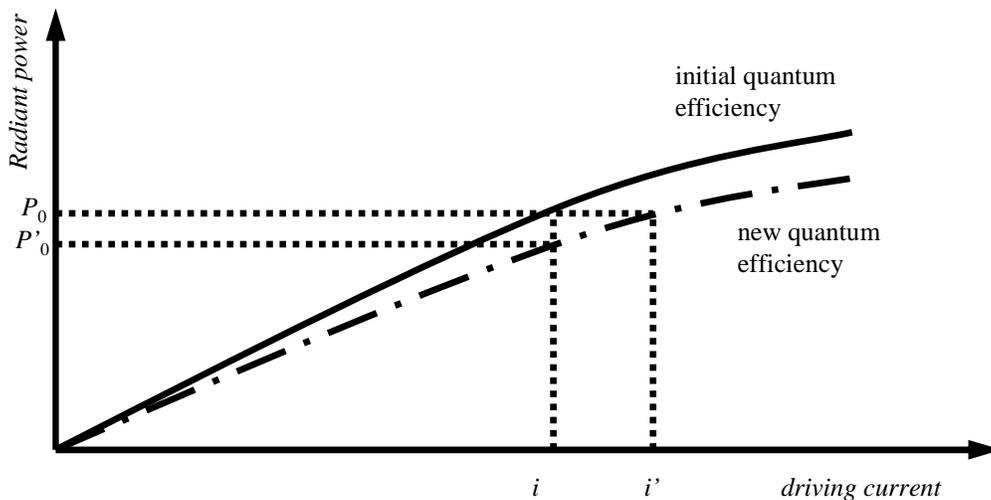
**Figure 2** – Characteristic curve of an LED (radiant power as a function of driving current) for two quantum efficiencies and ac driving currents.
