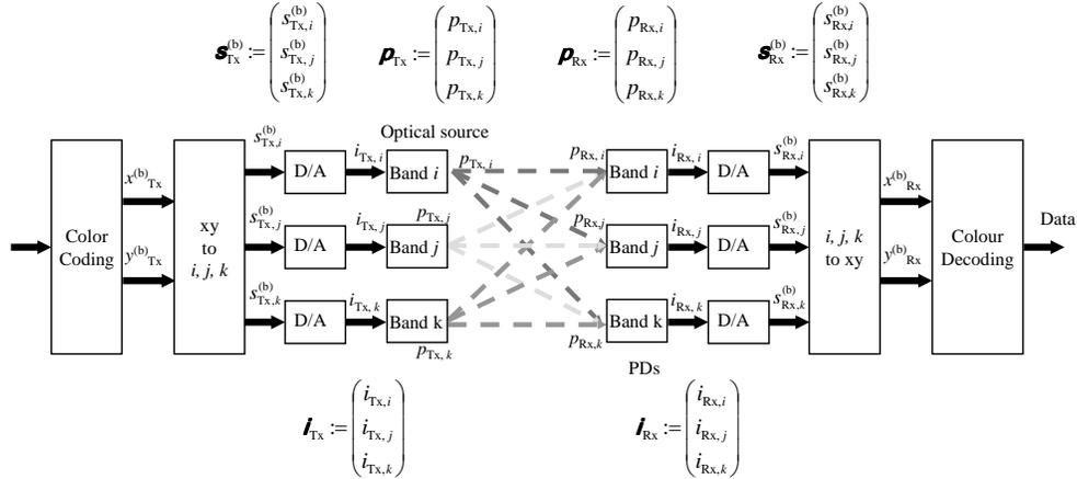
Figure 3 – Definition of system vectors and matrices for a CSK link.
