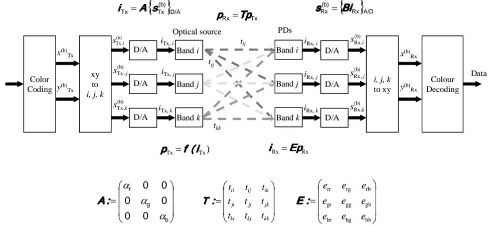
Figure 4 – Definition of further transfer matrices for a CSK link.
