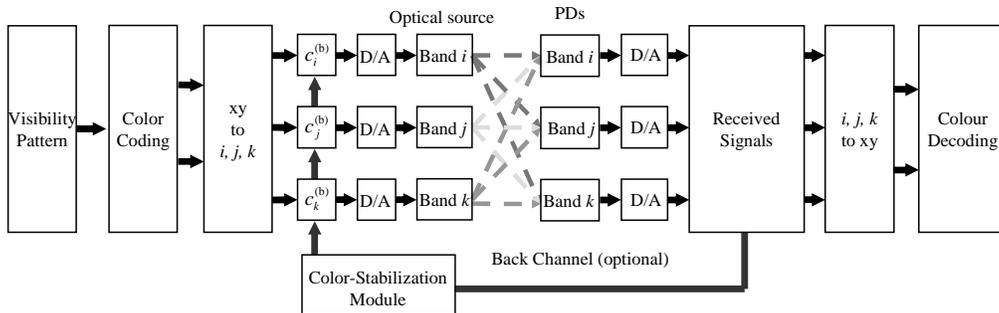
**Figure 5** – Detailed implementation of a color-stabilized CSK link. The received signals are relayed back to the transmitter, and the CSK receiver a channel-estimation module in the receiver estimates compensation factors and sends them back to the CSK transmitter via an additional channel.
