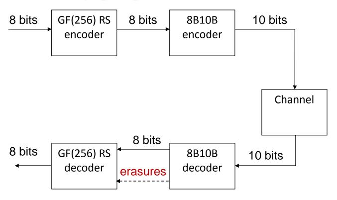
8b10b code naturally maps to the proposed (255,k) RS code since the code operates on GF(256), using 8 bits for a symbol
