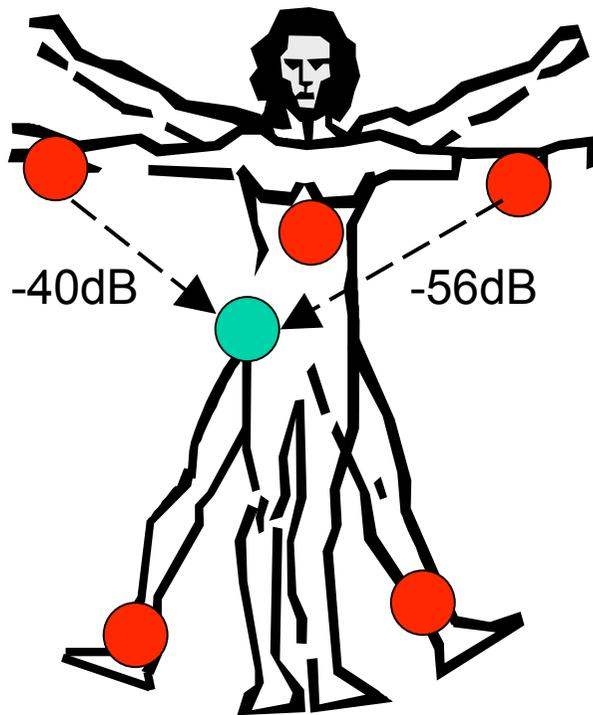
Wireless channel: Average path losses measured in testbed + **temporal variation** (parameters extracted from real testbed)
