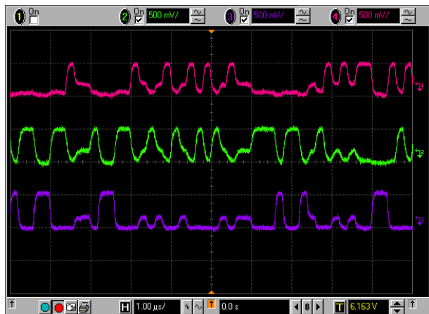
Demodulated Signal Symbol for CMC with symbol points (datadem)
