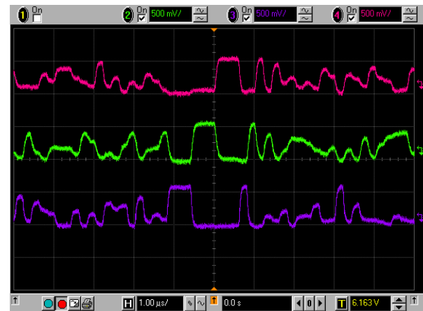
Demodulated Signal Symbol for CMC with symbol points (datadem)
