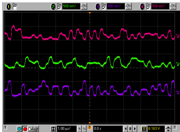
Demodulated Signal Symbol for CMC with symbol points (datadem)
