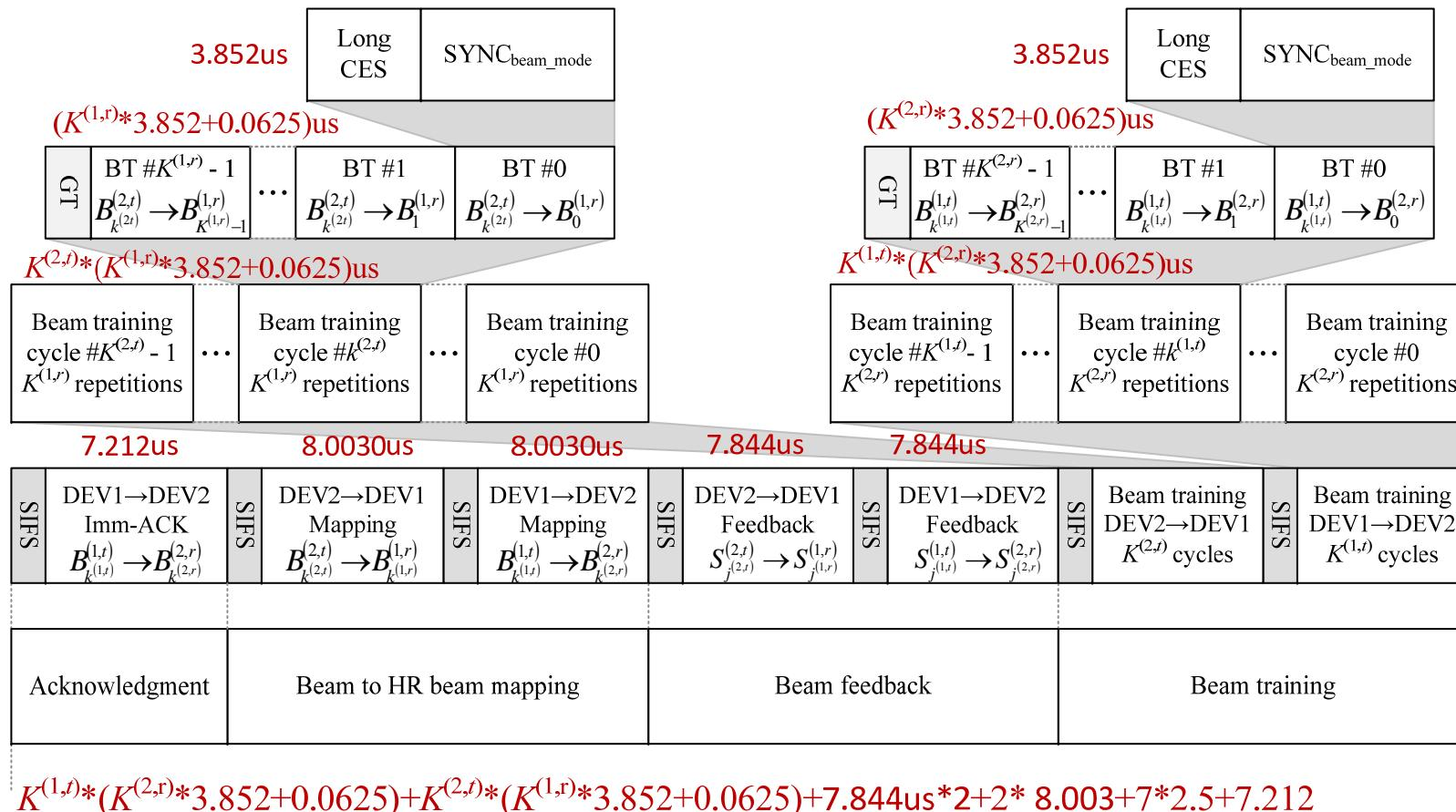
Maximum duration is 550.46us (maximum 8 beams per sector for both Tx and Rx of DEV1 and DEV2)
