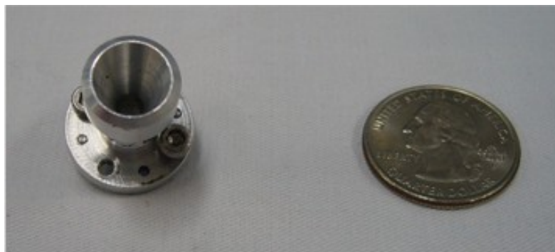
Conical horn antenna Beam-width 30 deg
