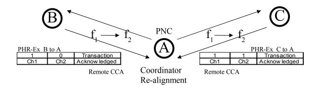
PNC is able to take action if sustaining No Acknowledged transaction on Node B. This may occur on a specific channel of Node B, or entire channel of Node B, and the information can be used to detect harmful Asymmetric Fault on the peer node.
