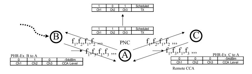
All nodes can take redundant opportunity to communicate on Ch.1 and Ch.2, and node B is getting interfered. PNC node A decides to switch channel by remote CCA and starts announcing the scheduled TX on Ch.1 and Ch.3. This alleviates the possibility of orphan generation.
