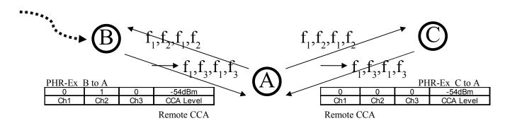
All TX node must follow the pre-defined TX channel order to send, in this case, AFA means alternating order. PNC node A is collecting remote CCA information and detect remote busy of node B on Ch.2.
