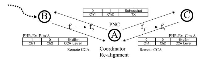
All node is using Ch.1 and node B is getting distracted due to interference, for example. PNC node A is collecting the remote CCA information from both node B and C periodically and detect the remote interferences at each node. If NHL decide to switch to alternate frequency channel of  $f_2$  i.e. Ch.2, in this case, conventional Coodinator Re-alignment can work. Before this decision of channel switch, PNC can use AFA-Ex of scheduled TX on Ch.2.
