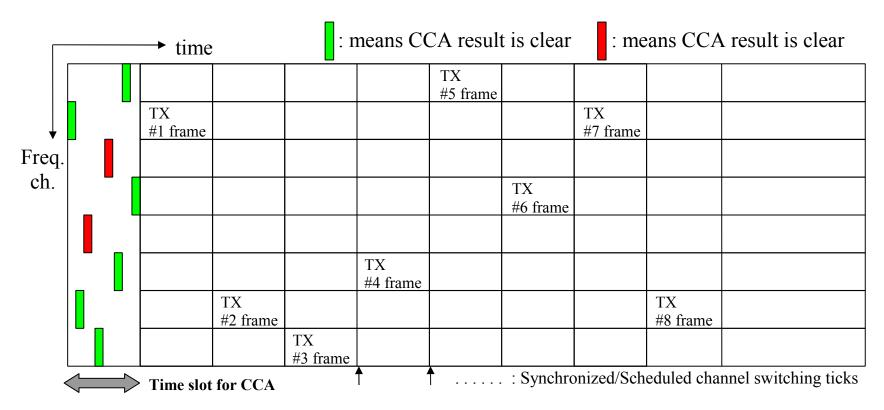
TX node must ensure at least a frame is following the previously scheduled channel and time slot unchanged to inform the new transmission channels and its order to send. Adaptive utilization of channels according to CCA is possible.
