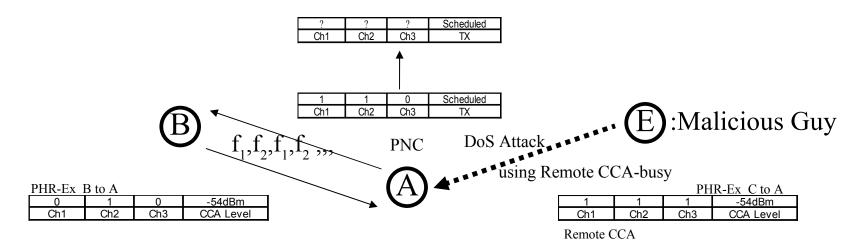
Although Node A and B can take account on node E's remote CCA busy, the credibility of node E itself and the authenticity of message pertaining this sort of remote busy may be verified through various ways, including simple statistical anomalies or usual masquerade detection.
