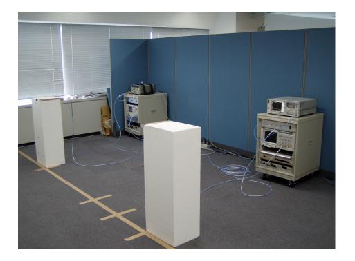
• It allows to implement arbitrary discrete UWB signals with a minimum sampling time of 0.1 nsec and 4 bits of resolution.
