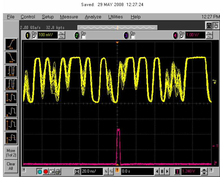
Wave form of received PN code
