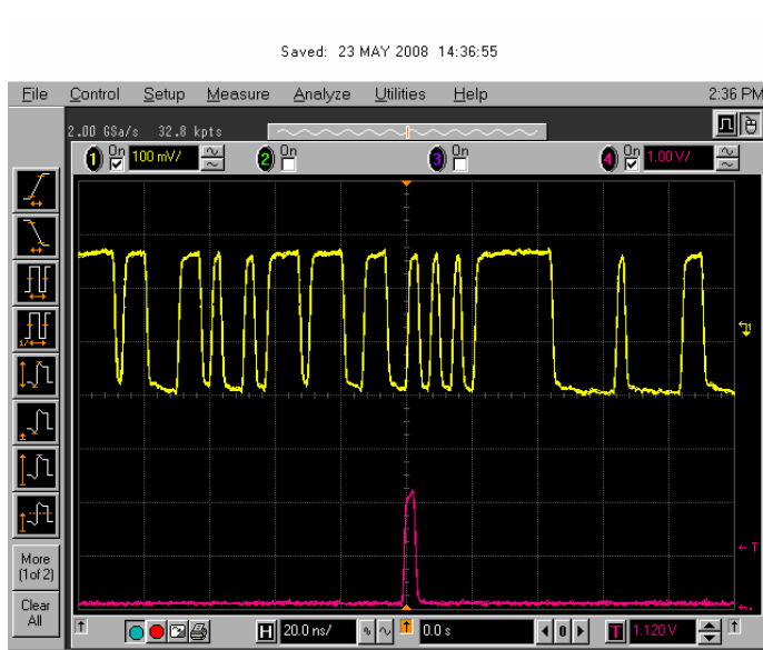
Wave form of received PN code
