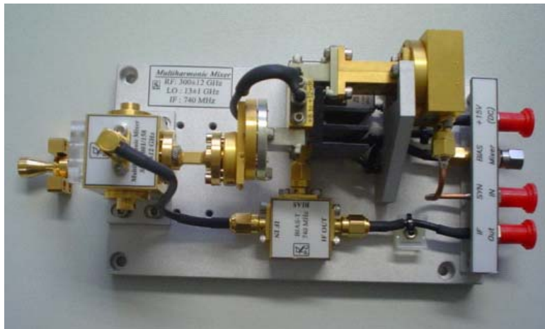
Receiver front end for 325 GHz in waveguide technology
