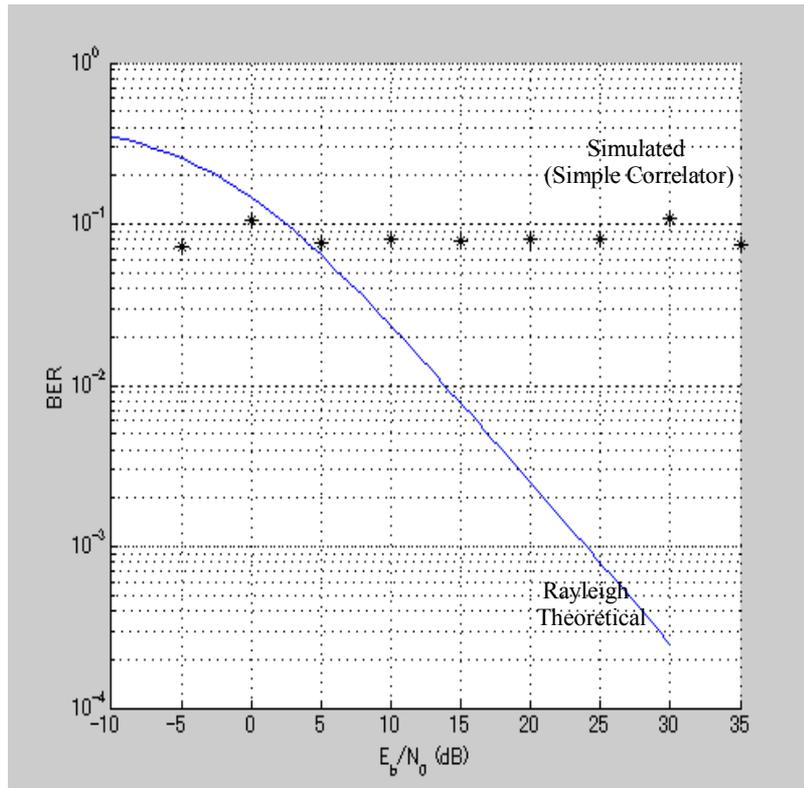
Because of 300kHz chip-rate, 3taps model with 1st tap of Rician  $k=12$ dB is substituted and used.
