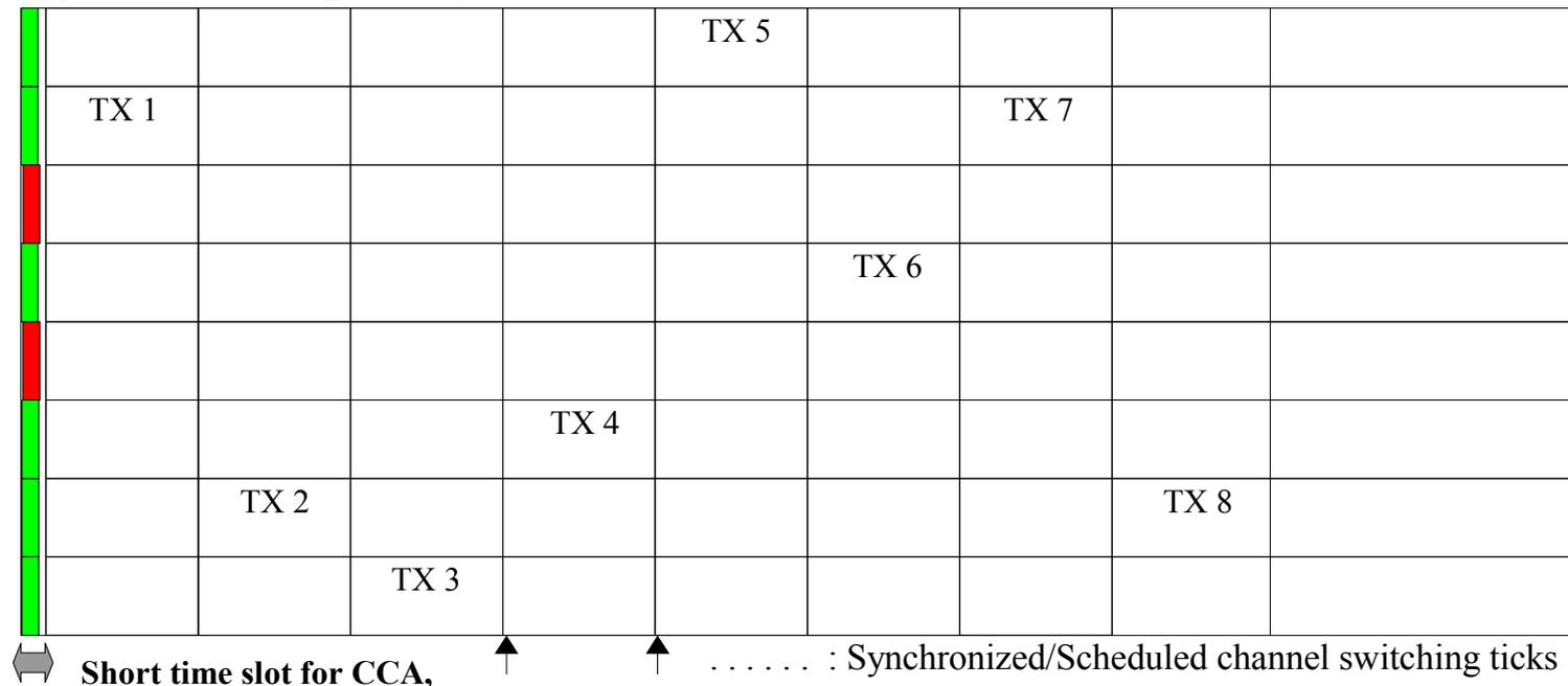
Even in this uncertain future scenario, TX node is supposed to include at least TX side information of channel usage by which RX node is able to be ensured if intended frame transmission have succeeded or failed. Simultaneous reception of multichannel at RX node would greatly improve the reliability of AFA.
