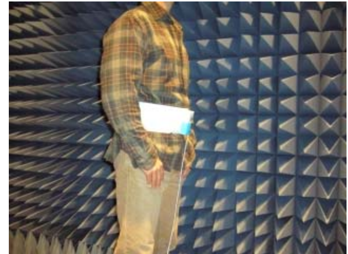
Skycross antenna on body f = 6.85 GHz
