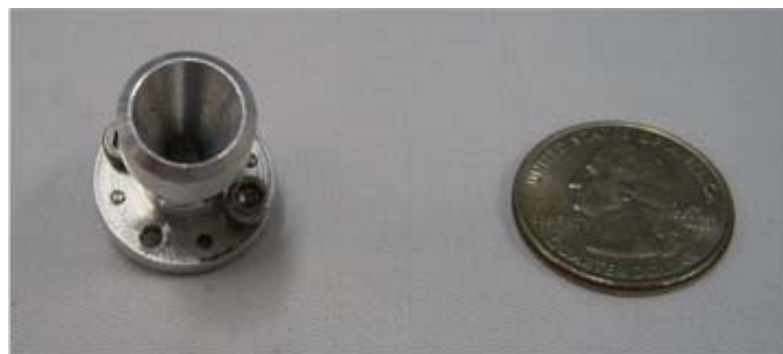
Conical horn antenna Beam-width 30 deg.
