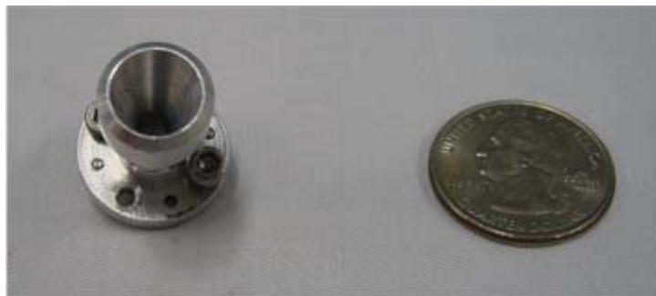
Conical horn antenna Beam-width 30 deg
